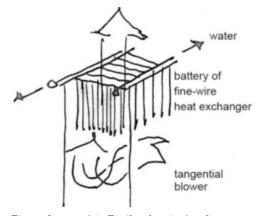
Figure 1: water/air Fiwihex heating/cooling
