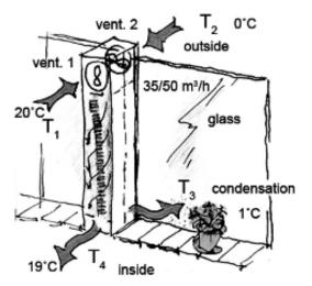
Figure 8: Operation scheme of a Breathing Window
