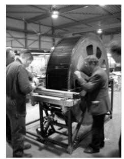
*Figure 4: The twinning machine for 1/10 mm fine wire heat exchanger in the breathing window*
