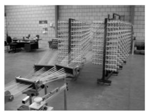
*Figure 3: The weaving of a 1/10 mm fine wire heat exchanger for very low temperature heating and cooling*
