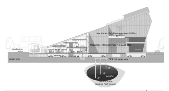
Figure 7: East façade cross section - Floriade 2012 world exhibition glasshouse - integrated design of 40.000  $m^2$  with an anearobic waste treatment and seasonal heat and cold storage in wet sand
